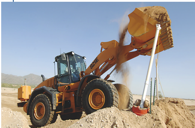
The 821E nears the top of the ramp used in the hopper-charging productivity study. The auxiliary fuel tank is at the right rear corner of the machine.
