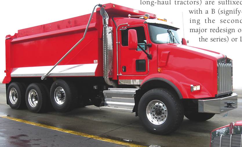
A setback steer axle identifies a T series truck, like this T800 dumper. It's got a Cummins ISM with an Allison automatic.
