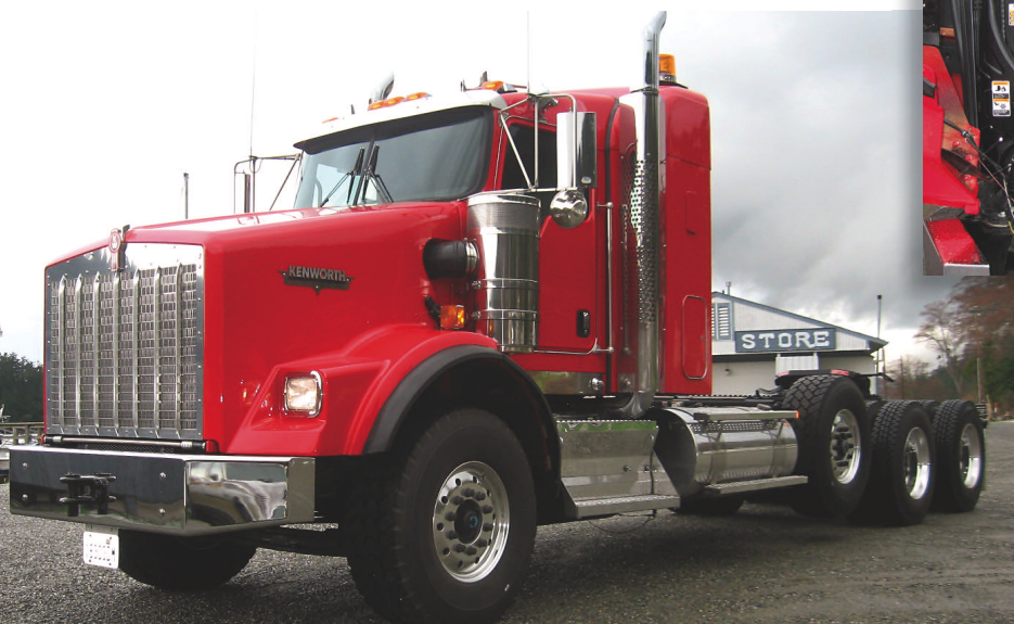
The T800H heavy haul tractor looks impressive just sitting there, even without a loaded trailer. Its wide hood houses a big, high-capacity radiator and (inset) 600-hp Cummins ISX.
