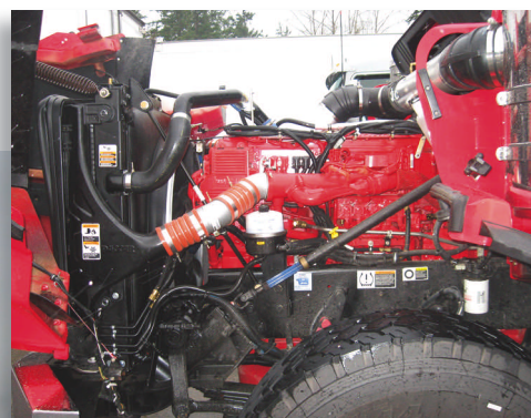
The T800H heavy haul tractor looks impressive just sitting there, even without a loaded trailer. Its wide hood houses a big, high-capacity radiator and (inset) 600-hp Cummins ISX.
