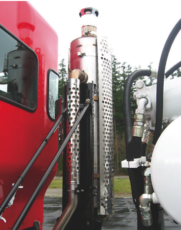
Stack on the Cat-powered W900S includes the big diesel particulate filter, which looks like and doubles as a muffler, with a Clean Air Induction pipe that leads from the DPF back to the engine.
