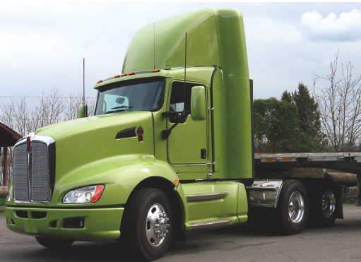
Third T model in our trio is this T660 Extended Day Cab tractor, which would give cargo on the flatbed trailer, not to mention its driver, a smooth ride. It's got a Cat C13 with an Eaton UltraShift.
