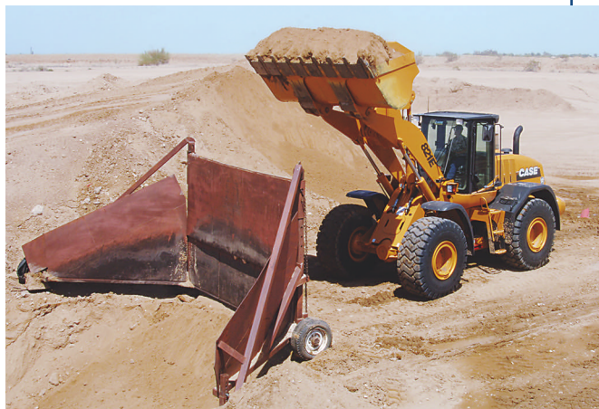
The 821E prepares to dump over the "truck" in the short-cycle loading test.
