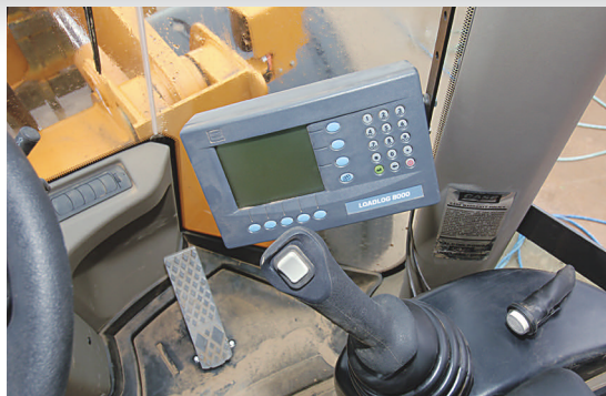
During the evaluation, material weights were recorded by an RDS LOADLOG 8000 on-board weighing system, which provided a cycle-by-cycle printout of results.
