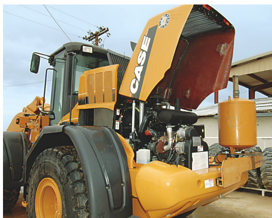
The 821E's tilt-up hood (electrically raised) provides wide-open access to routine maintenance points. Removable inner fenders below the hood further increase service access, as do pull-up side sheets (forward of the hood) and a tilt-up panel above the cooling module.
